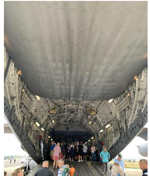
The cargo area of a C17 Transport Plane, which can carry a Chinook Helicopter. In the 2021 Afghanistan evacuation, over 400 passengers a time were airlifted to Dubai
