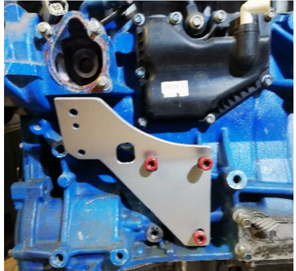
Custom Engine Mounting bolted to Duratec Engine
