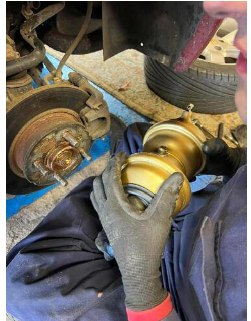
Remanufactured spheres being fitted
