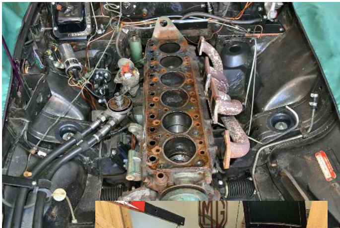
Top: Head removed and progress being made
