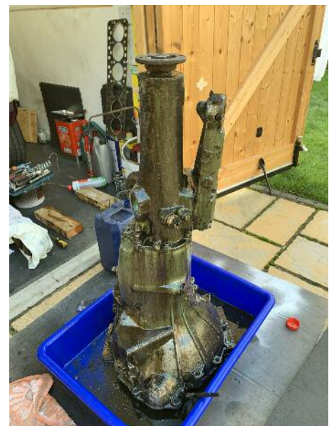
Right: One of the muckiest jobs around. Cleaning off years of oil and road gunk
