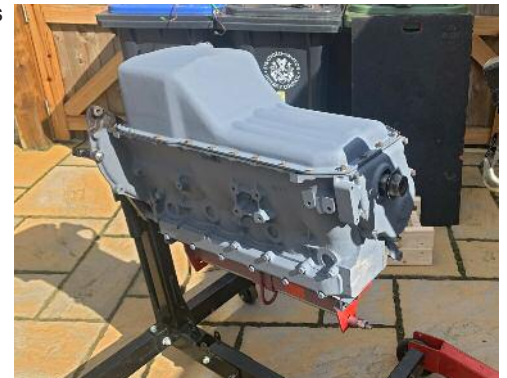
Sump finally in place – hope this doesn't have to come off again in a hurry
