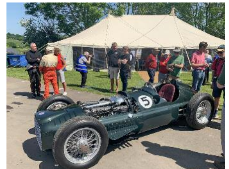
Prescott - The V16 1500cc Supercharged 600bhp BRM - Rob Hall is far left.
