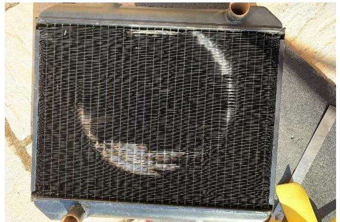
Cooling fan leaving its mark
