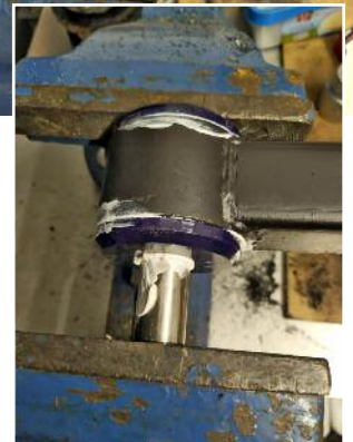
Photograph 7 - The smaller bush being pressed in using a socket to accommodate the bush passing through the angle piece.
