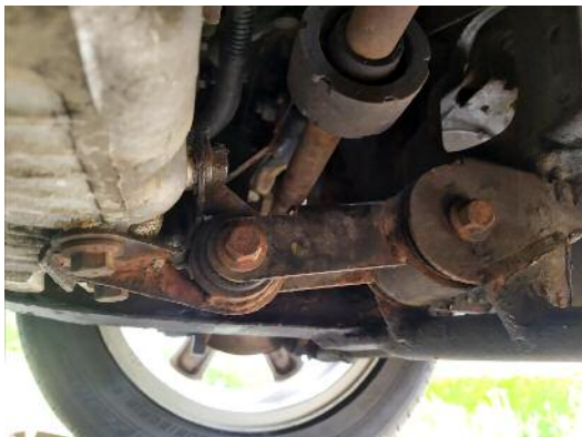
Photograph 1 - The before shot showing the tie-bar. It is in two pieces. An angled part (smaller bush) fitted to the sump with 4 bolts and a straight part (larger bush) connected to the subframe. All bolts have 15mm heads. The bolt running through the subframe, and larger bush, is a struggle to extract because of its
