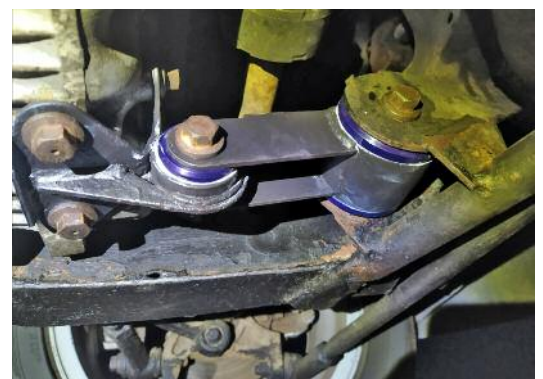
Photograph 4 - The new bushes, 'crush tubes' and lubricant.
