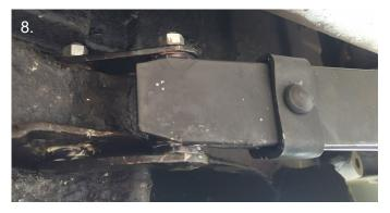
Tighten all nuts to remove the slack, fit road wheel, and lower to the ground before tightening completely. Enjoy the new driving experience.
