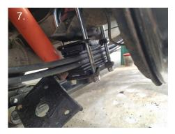
Next, fit the front bolt. Again, jostling will be required to align the fixing points with the front eye of the spring. Screwdrivers/drifts, etc are useful but I used an old bolt ground to a bullet point at the end. Do not forget to use plenty of copper grease. Put the washer and nut on but keep it loose.
