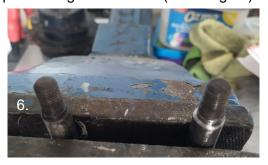
Using the drum jack to adjust the height, offer up the centre of the parabolic spring, with poly pads and brackets fitted, and fit the U-bolts and nuts. This is fiddly and the use of bricks can be recommended to support the spring whilst jostling into position. DO NOT TIGHTEN THE U-BOLT NUTS! Keep it slack (see image 7).
